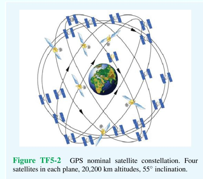
Figure TF5-2 GPS nominal satellite constellation. Four satellites in each plane, 20,200 km altitudes,  $55^\circ$  inclination.
